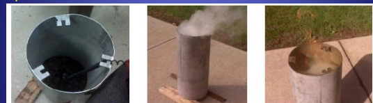
Thermometer → Smoke in 24 Minutes → Fire in 32 Minutes
